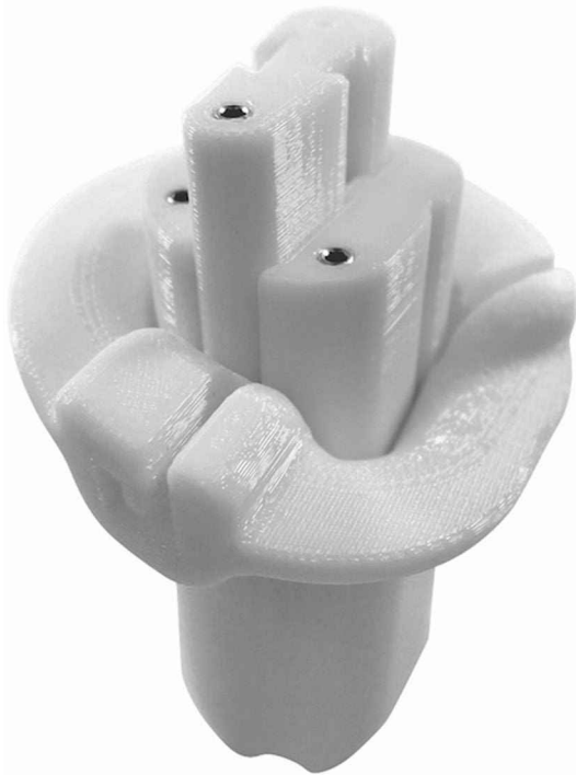
Fig. 6 A patient-specific tubular retractor for a minimally invasive transforaminal lumbar interbody approach that is designed to match the tissue depth and contours of this patient’s posterior L5–S1 bony anatomy. The retractor is secured to the spine using a cannulated bone screw along the trajectory of the existing S1 pedicle screw
