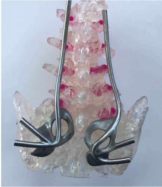
Fig. 4 1:1 scale biomodel of patient’s spine with patient-specific 3D-printed titanium implants contoured to match the bony anatomy of the pelvis and desired spinal curvature for revision surgery
