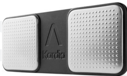
Fig. 9.3 KardiaMobile EKG Monitor from AliveCor, capable of measuring heart rhythm in conjunction with a smartphone
